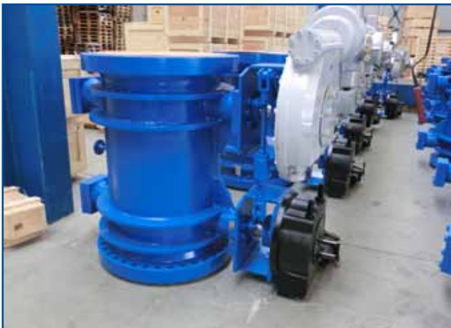
30" Class 300 DBB with electric actuator as master device and declutchable gear box.
